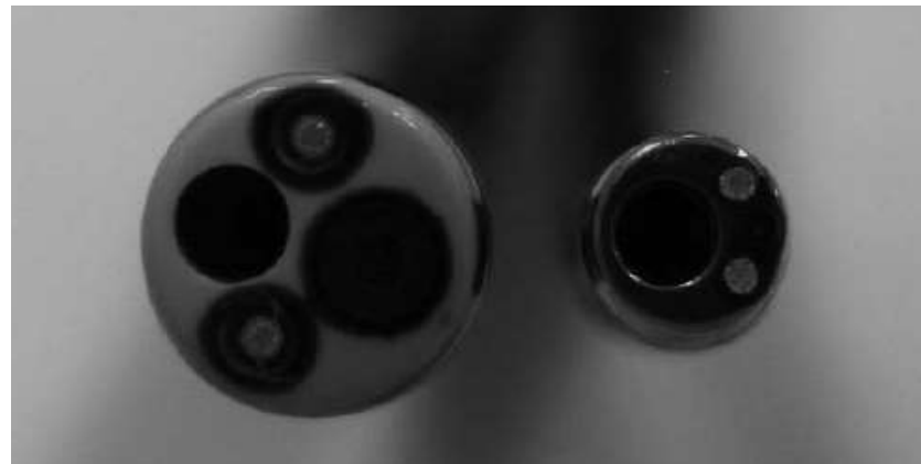
Thin 3.5 mm bronchoscope 1.7 mm working channel
