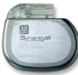
1989 Dual chamber rate response Synergist
