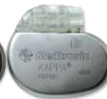
1998 Rate response via activity & minute ventilation Kappa®
